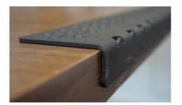
2. Starting with the middle screw holes, drill your screws into the stair working your way out from the center. Make sure that you are drilling perpendicular to the surface and that you use all of the screw holes provided. Installation is complete once all screws have been drilled into place. Note that the screw holes are not raised; <u>DO NOT use the raised traction bumps for your screw placement.</u>
