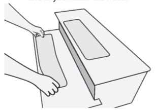
Make sure to push out any bubbles from under the tread.
