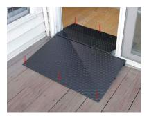
STEP FIVE: Place the Ramp Pieces **Together** - The crossover bridge moves down on its hinge to create a platform from the outdoor ramp to the indoor ramp. The crossover bridge will rest on the lip of the indoor ramp when in use. For your safety, we recommend securing both the outdoor and indoor ramps to the floor using screws through the predrilled holes on the ramp (see arrows).
